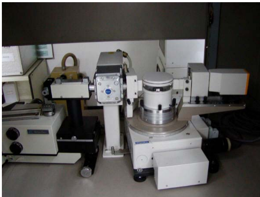
Figure 3.3 XRD Rikagu RINT 2000 at PPC.
