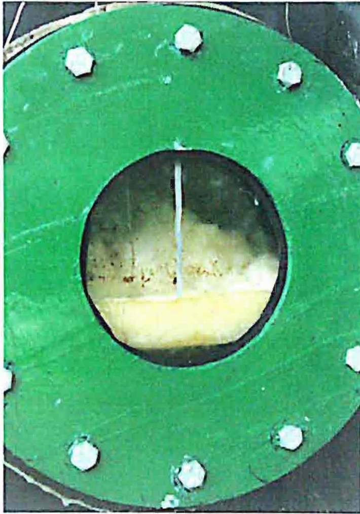
C.9 Produced ice in the storage tank
