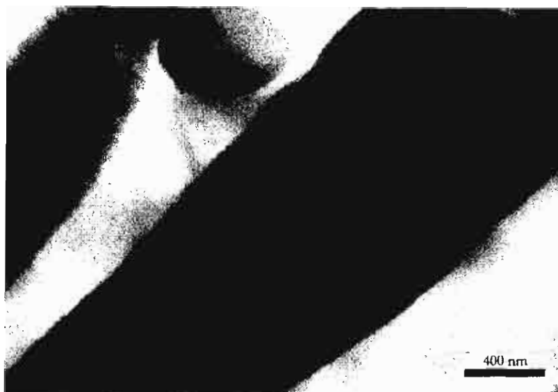
Figure 3. TEM micrograph showing the detail of the morphology of a PP sample containing 40 wt% of EcO 2 . The sample was mixed in an internal mixer, sheared between parallel plates at 230°C, and then quenched. Micrograph shows a section taken at 5 mm from the center of the sample; at this position, shear rate was 10 s -1 .
