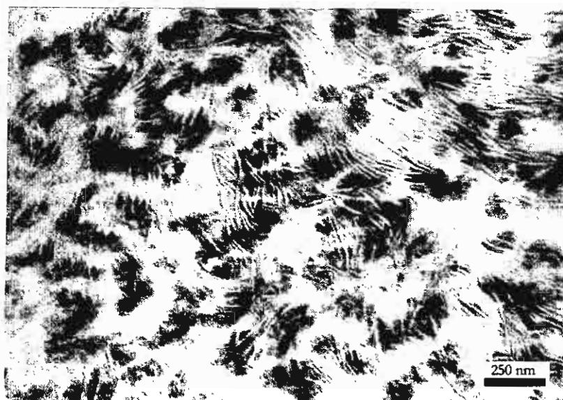
Figure 5. TEM micrograph showing the interpenetrating morphology found in the PE1 specimens, molded at 230°C and 0 Pa back pressure, containing 27.9 wt% of EcO2.
