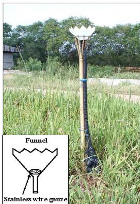
Fig 1. The photograph of an air particulate collector.
