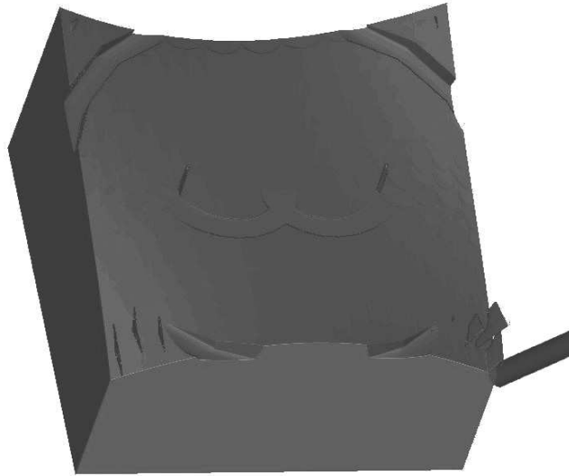
Fig. 2.13. Cutting simulation of surface in Fig. 2.11 with 20 \times 20 tool path
