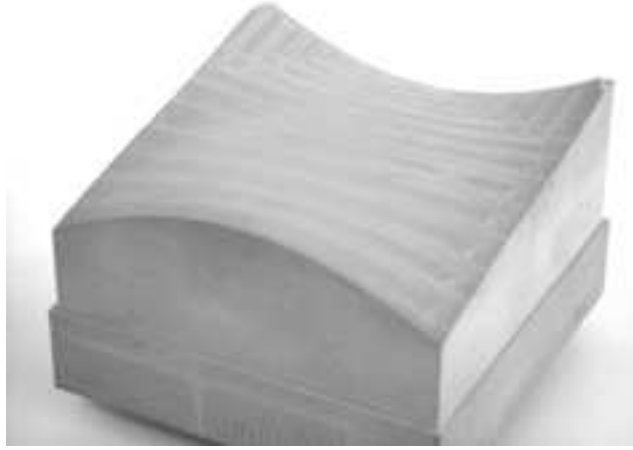
Fig. 4.13. Practical machining using the SFC tool path with correction
