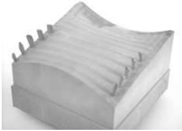
Fig. 4.12. Practical machining using the SFC tool path without correction
