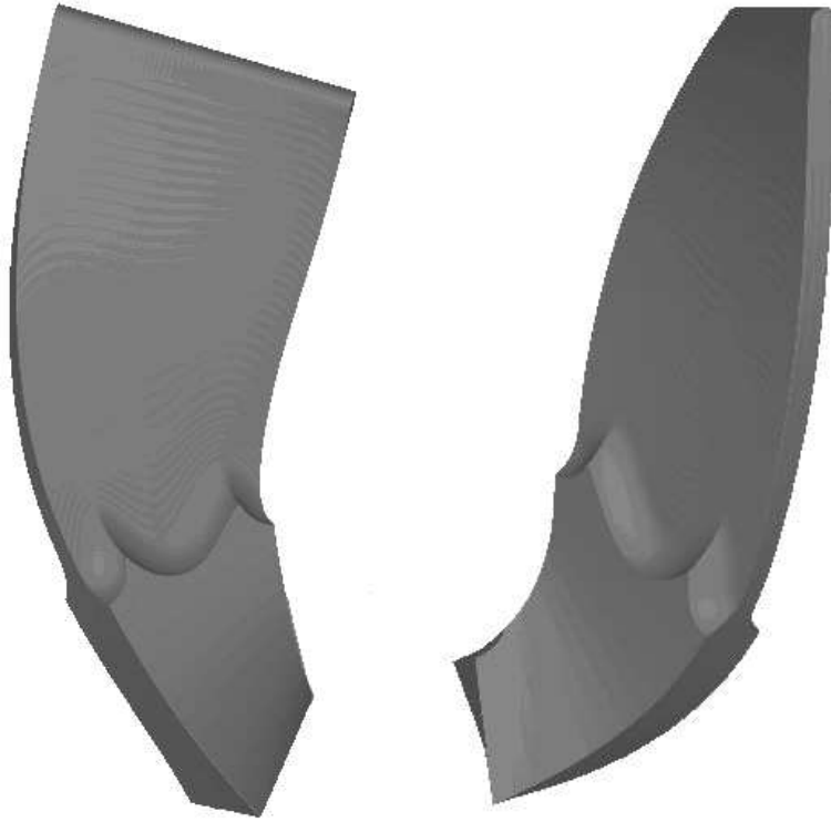
Fig. 5.33. Virtual cutting of the blade in Unigraphics 18
