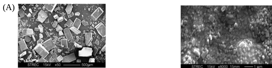
Figure 2 SEM microphotographs of (A) conventional suspension, and (B) nanosuspensions prepared by precipitation-lyophilization-homogenization (PLH) method of clarithromycin formulation (14).
