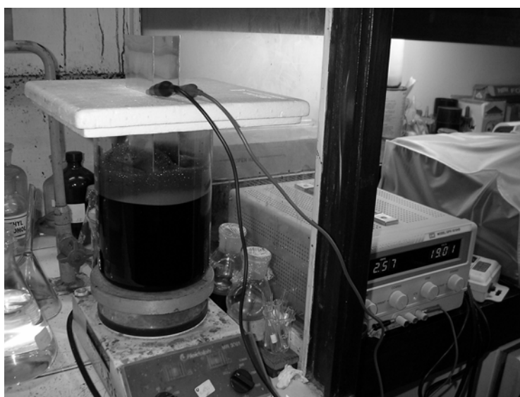
Figure 1. A typical electrocoagulation setup.
