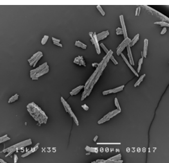
Figure 35 SEM photomicrographs of dehydrated pentahydrate NF during isothermal dehydration after the complete dehydration with respect to T_{iso} (left column at the magnification of 35, right column at the magnification of 5000)
