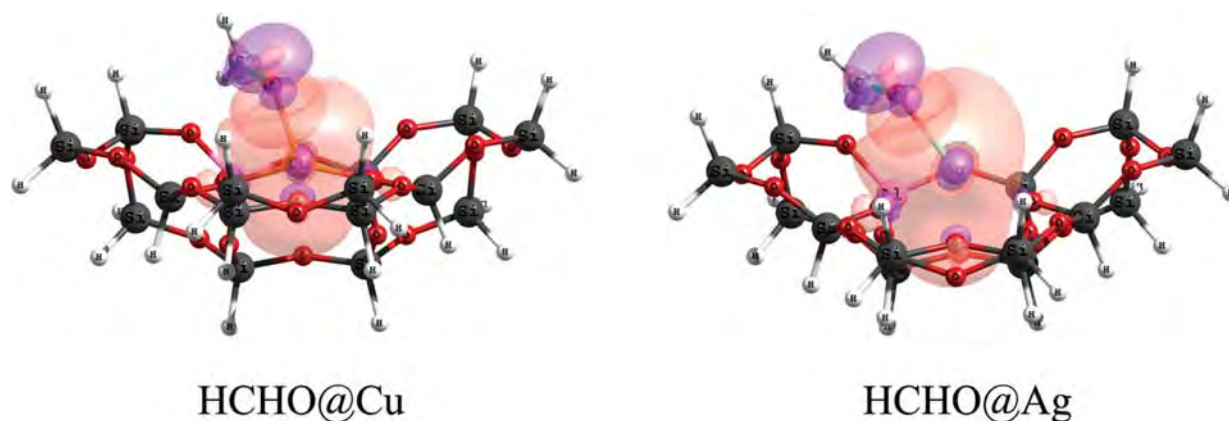
Figure 4. Illustration of the interaction between the 2p orbital of formaldehyde and the 4s orbital of Cu (left)/the 5s orbital of the Ag (right), analyzed from the NBO calculation with the M06-L/6-31G(d,p) method. The isosurface value is \pm 0.03 au.
