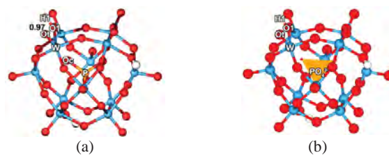
Figure 2. Cluster model of \alpha -Keggin HPW heteropoly acid: (a) atomistic graphics with the acidic bond distance and (b) an orange tetrahedron representing the phosphate anionic core of the HPW.
