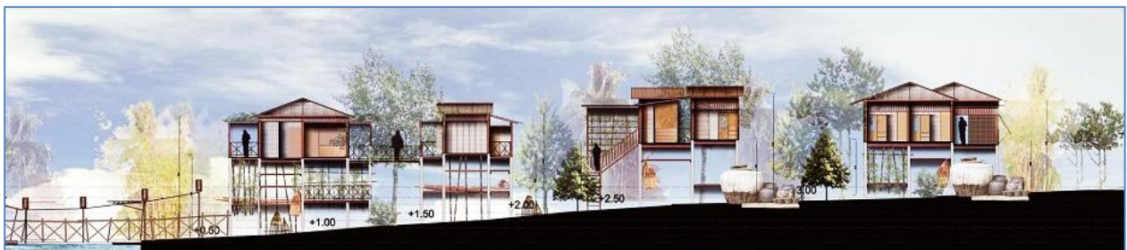
Figure 3.37 Adaptability of housing floors in response to levels of flood water
