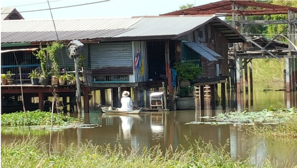
Figure 5.25: Stilt houses reflects unique way of living as commonly seen in and around Ban Rangnok flooding mitigation approaches. A new coming house which has been elevated in higher level (Right) compared to the Existing stilt house (Left).
