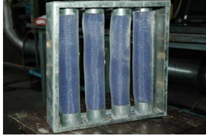
Figure 3: A media column containing of silica gel 0.75 kg
