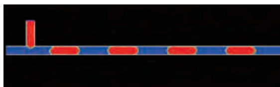
Fig. 1 The simulated Taylor flow in microchannel ( U_G = 0.0694 m/s, U_L = 0.0764 m/s)
