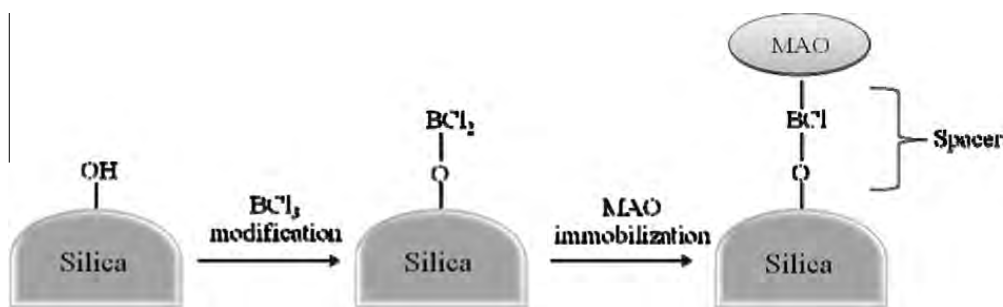
Scheme 2. Conceptual model for \text{BCl}_3 effect as a spacer.
