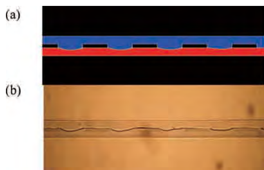
Fig. 5 (a) The simulated stable two phase flow pattern with Model A at 0.0148 s and (b) experimental observation
