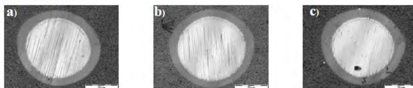
Fig. 1: Optical micrographs of Calotest on samples coated at different nitrogen pressures a) 2 Pa, b) 1.5 Pa, and c) 1 Pa.
