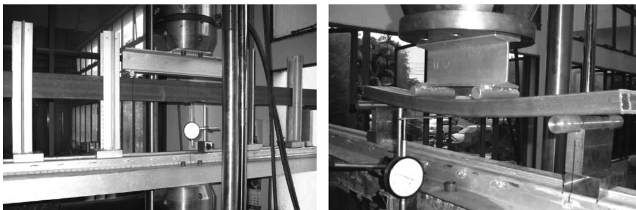
FIG. 2. An experimental arrangement for four-point bending tests for WPVC-1-test specimen in edge-wise and flat-wise directions for WPVC composite. [Color figure can be viewed in the online issue, which is available at www.interscience.wiley.com .]
