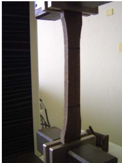
Figure 4 Typical setup of tensile test
