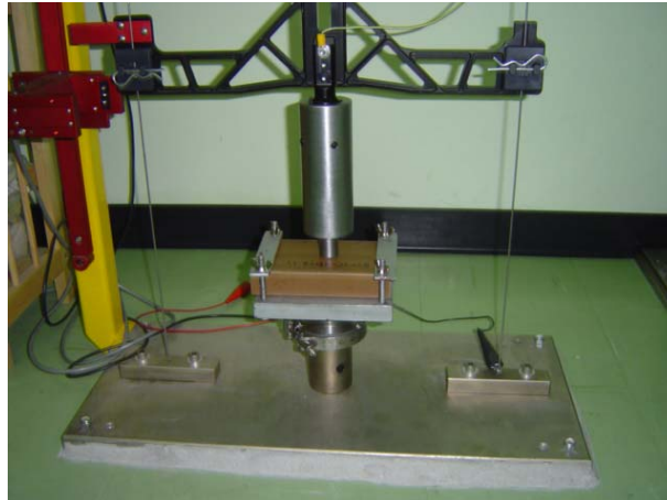
Figure 5 Typical setup of impact test
