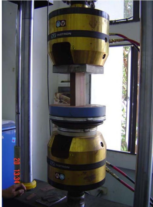
Figure 6 Typical setup of compression parallel-to-extrusion test
