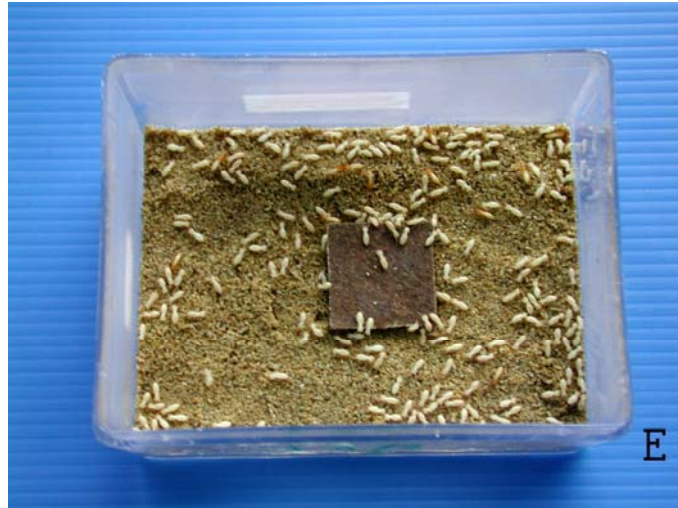
Figure 14 Typical setup of termite resistance test
