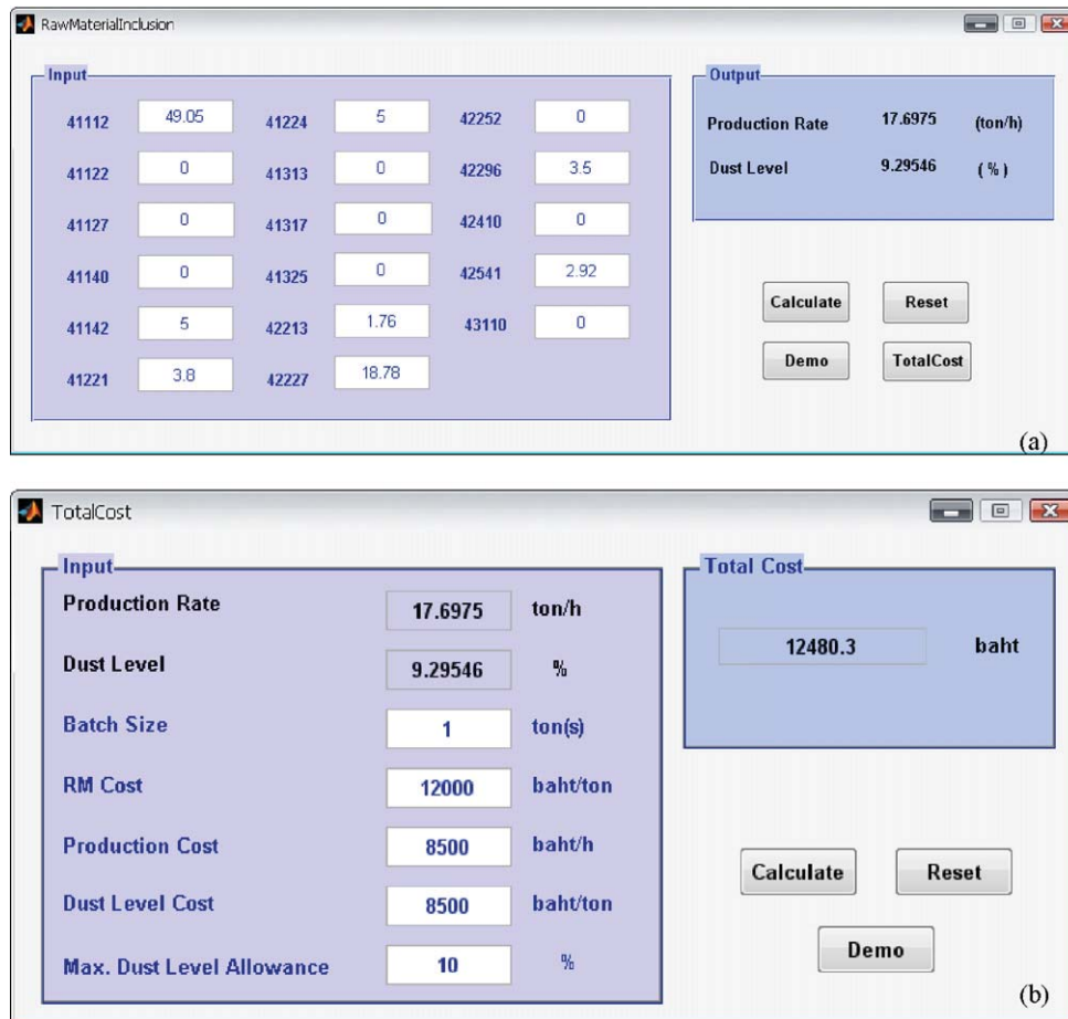
Fig. 3. Graphic user interface showing its results of production rate and dust level prediction (a) and estimation of total cost (b).
