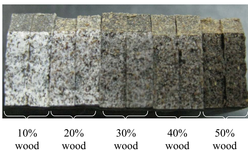
Figure 6.23: Fracture surface of PVC/ABS(SP200)/wood composites at a fixed PVC/ABS mass ratio of 50/50 at various woodflour contents.
