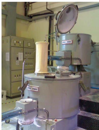
Figure 5.1: High speed mixer: Plasmec Turbomixer 100 litres with a cooler for PVC dryblend preparation.
