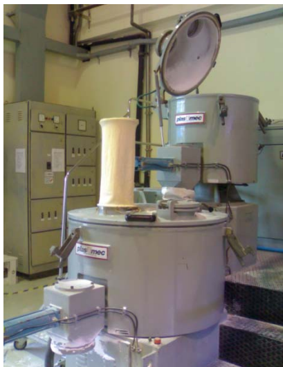
Figure 11.1: High Speed Mixer: Plasmec Turbomixer 100L with cooler (made in Italy).
