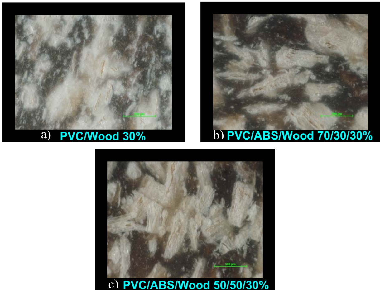
Figure 6.36: Optical micrographs showed the surface of the specimens after 50 days exposure at a fixed 30 wt% woodflour loading with various matrix: a) PVC/wood composite b) PVC/ABS wood composite at 70/30 mass ratio c) PVC/ABS wood composite at 50/50 mass ratio
