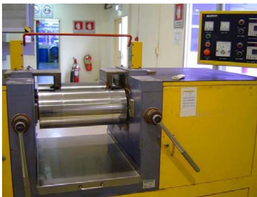
Figure 5.2: Two-roll mills for PVC/ABS blends preparation (Lab Tech).
