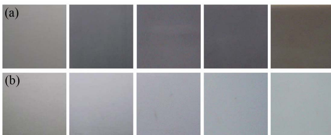
Figure 12.13a: Visual appearance of the sample surfaces after weathering at various outdoor exposure time: a) PVC b) PVC/ASA 50:50 wt%.
