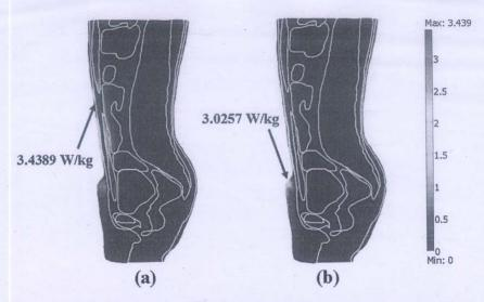
Fig. 9 SAR distribution in human body (W/kg) exposed to the leakage power density of 5  $\,$  mW/cm² at the frequencies of (a) 915 MHz and (b) 2450  $\,$  MHz
