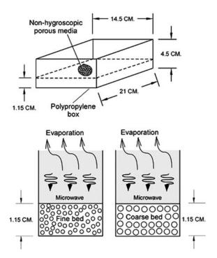
FIG. 2. Schematic of drying sample (porous packed bed).
