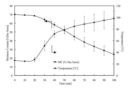
Figure 4.12 Temperature and moisture variations versus elapsed times in case drying using CMCB ( $T_1$ = hot air 70 °C)( case 9:Top feed)
