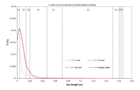
Fig. 5.12 Temperature distribution versus arc-length of the human body at various times exposed to the electromagnetic frequency of 2,450 MHz at the leakage power density of 5 mW/cm<sup>2</sup>
