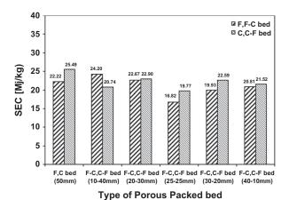
Fig. 16. Variation in specific energy consumption under microwave and convective drying at drying time 240 min.
