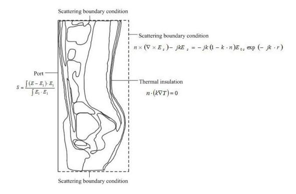
Fig. 5.3 Boundary condition for analysis
