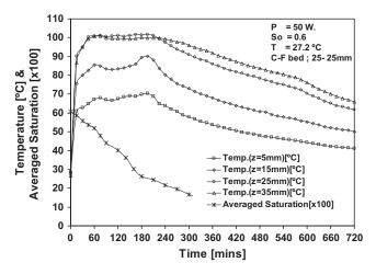
**Fig. 13.** Temperature and averaged saturation profiles with respect to elapsed time (C–F bed, depth 25–25 mm).
