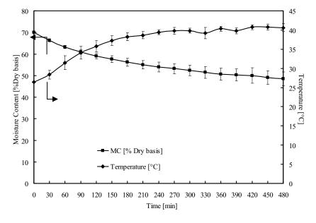
Figure 4.13 Temperature and moisture variations versus elapsed times in case using convective drying ( $T_1$ = hot air 70 °C)( case 10)
