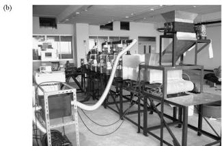
Fig. 1. Experimental equipment: continuous microwave belt drier.
