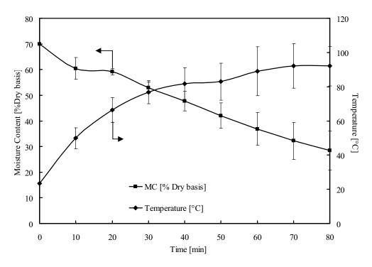
Figure 4.6 Temperature and moisture variations versus elapsed times in case drying using CMCB ( $T_1$ = Ambient 30 °C)( case 3:Top feed)
