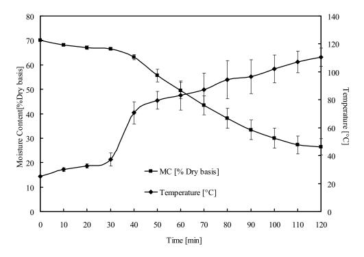
Figure 4.8 Temperature and moisture variations versus elapsed times in case drying using CMCB ( $T_1$ = hot air 70 °C)( case 5:Top feed)
