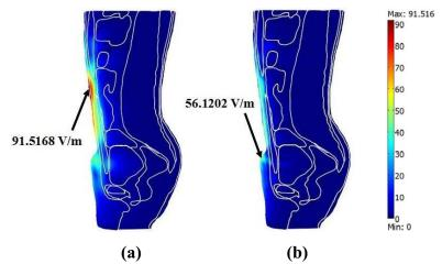
Fig. 5.8 Electric field distribution in human body (V/m) exposed to the leakage power density of 5 mW/cm<sup>2</sup> at the frequencies of (a) 915 MHz (b) 2,450 MHz
