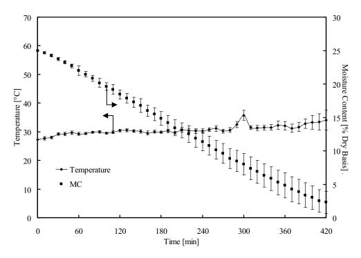
Figure 3.9 Temperature and moisture variations versus elapsed times in case using a convective drying ( $T_1$ = 70 °C)( case 8,F-bed)
