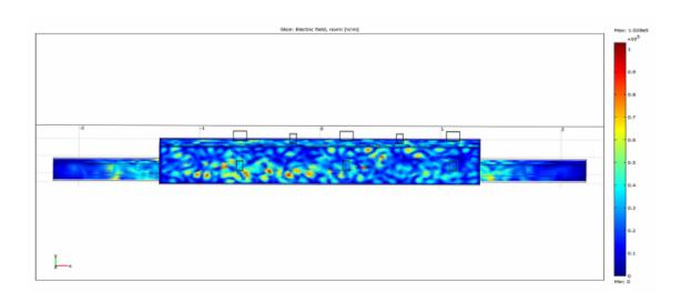
Computer simulation of electromagnetic field inside multi-mode cavity
