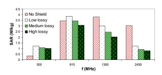
Fig. 6.9 Comparison of the maximum SAR in human model at the frequencies of 300MHz, 915 MHz, 1,300MHz and 2,450 MHz
