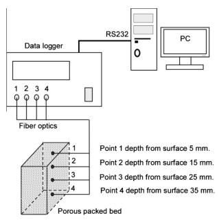
Fig. 2. Temperature measuring.
