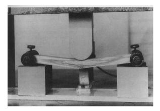
Fig. 10. BSI Standard of static bending test of specimen [31].
