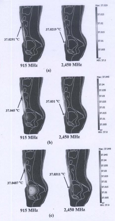
Fig. 10 The temperature distribution of human body exposed to electromagnetic wave at the frequencies of 915 MHz and 2450 MHz: (a) 1 min, (b) 10 min, and (c) steady state
