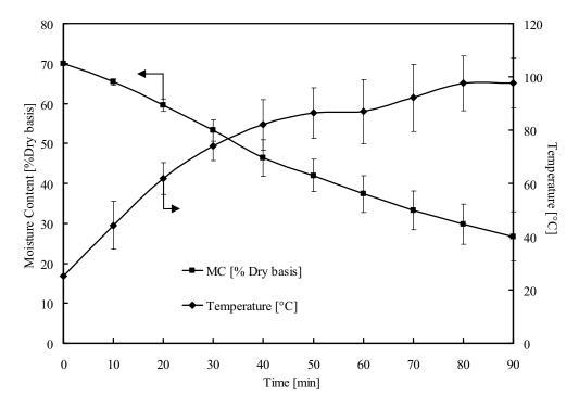
Figure 4.7 Temperature and moisture variations versus elapsed times in case drying using CMCB ( $T_1$ = Ambient 30 °C)( case 4 : Screw feed)
