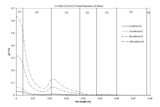
Fig. 5.18 Temperature increase versus arc-length of the human body exposed to the electromagnetic frequency of 915 MHz at various leakage power densities, at t=1min
