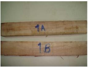
Sample before dried with Combined Multi-Feed Microwave -Convective Air and Continuous Belt System (CMCB)
