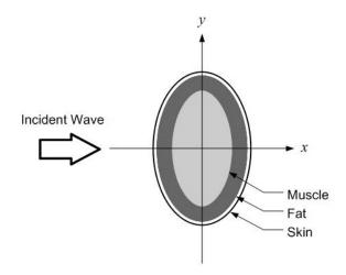
Fig. 6.6 Geometry of the validation model (Nishizawa and Hashimoto, 1999)
