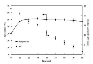
FIG. 4. Temperature and moisture variations versus elapsed times in case drying using CMCB ( $T_1=30^{\circ}C$ ) (C-bed, case 1).
