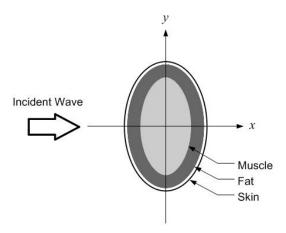
Fig. 5.6 Geometry of the validation model obtained from the previous work (Nishizawa and Hashimoto, 1999)
