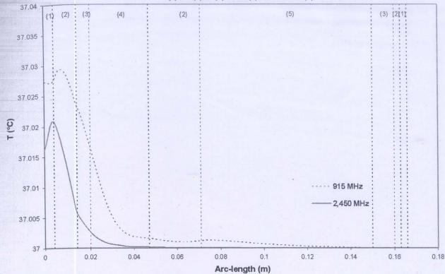
Fig. 15 Temperature distribution versus arc length of the human body exposed to the leakage power density of electromagnetic field at 5 mW/cm<sup>2</sup>
