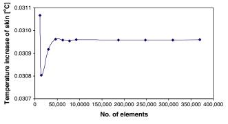
Fig. 5. Grid convergence curve of the 2D model.
