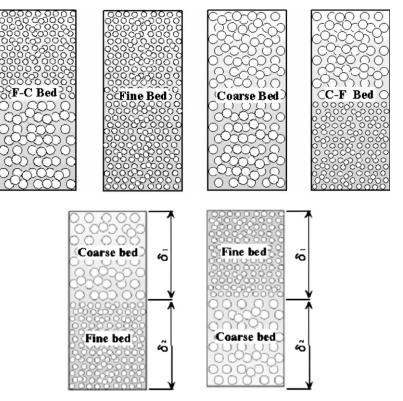
Fig. 3. Multi-layered porous packed bed (sample).
