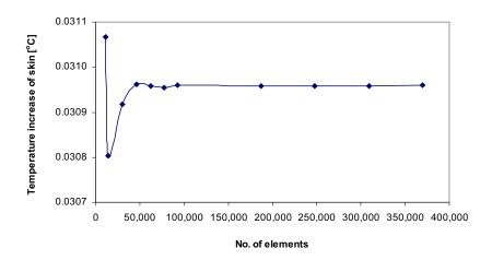
Fig. 5.5 Grid convergence curve of the 2D model
