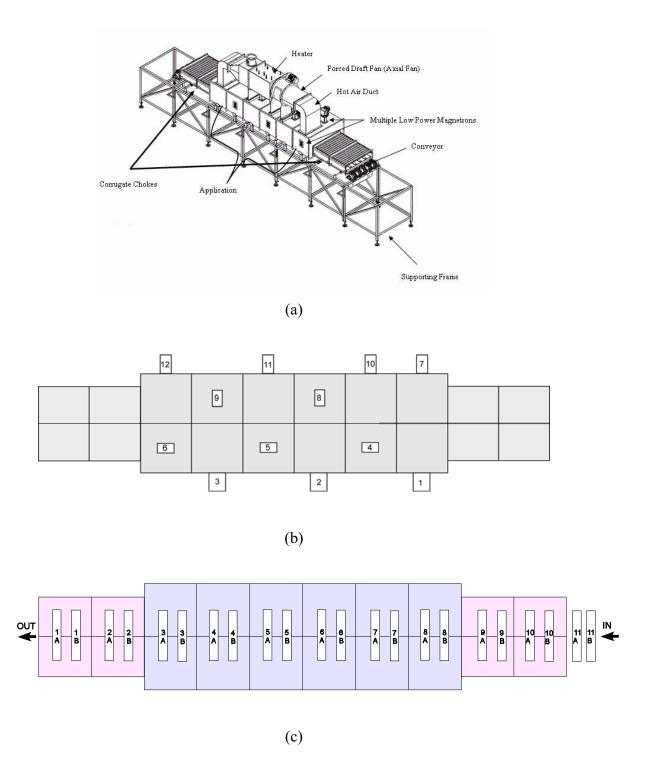
Figure 4.1 Schematic diagram of experimental set up
