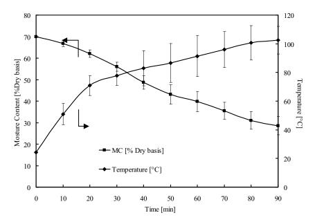
Figure 4.5 Temperature and moisture variations versus elapsed times in case drying using CMCB ( $T_1$ = 70 °C)( case 2 : Screw feed)
