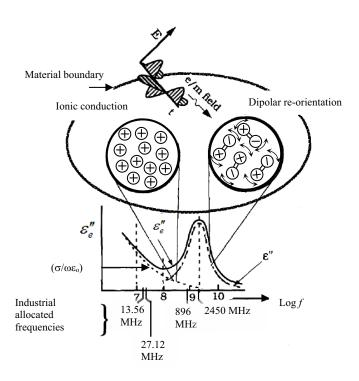
Figure.1.3 Effective loss factor due to dipolar ionic conduction
