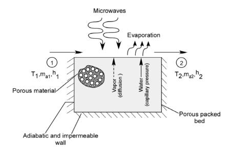
Figure 1.6 Microwave and convective drying process.
