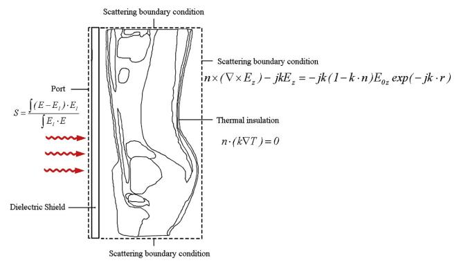
Fig. 3. Physical model and boundary condition used for analysis.
