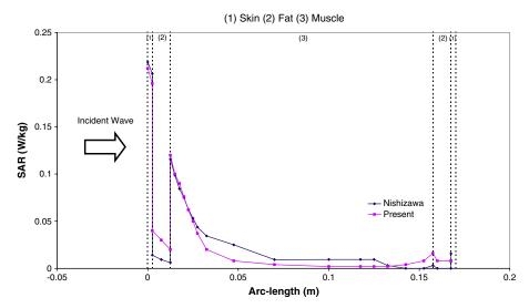
Fig. 7. Comparison of the calculated SAR distribution to the SAR distribution obtained by Nishizawa et al. [9].
