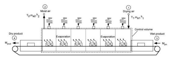
FIG. 3. Schematic of control volume representing drying process using a combined multi-feed microwave-convective air and continuous belt system (CMCB).
