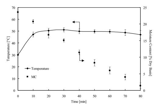
Figure 3.4 Temperature and moisture variations versus elapsed times in case drying using CMCB ( $T_1$ = 30 °C)( case 1,C-bed)
