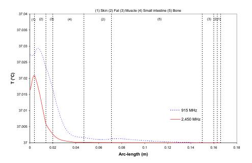
Fig. 5.15 Temperature distribution versus arc-length of the human body exposed to the leakage power density of electromagnetic field at 5 mW/cm<sup>2</sup>
