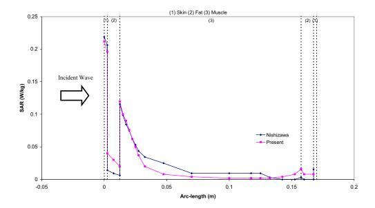
Fig. 5.7 Comparison of the calculated SAR distribution to the SAR distribution obtained by Nishizawa et al. (Nishizawa and Hashimoto, 1999)
