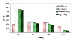
Fig. 6.10 Comparison of the maximum temperature increases in human model at the frequencies of 300MHz, 915 MHz, 1,300MHz and 2,450 MHz
