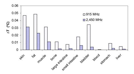
Fig. 5.17 Comparison of the temperature increases in human tissues at the frequencies of 915 MHz and 2,450 MHz.
