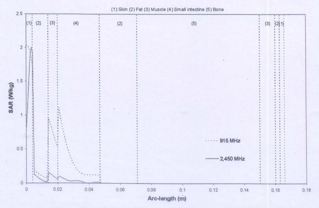
Fig. 14 SAR distribution versus arc length of human body exposed to the leakage power density of electromagnetic field at the 5 mW/cm<sup>2</sup>
