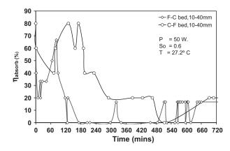
Fig. 11. The variation of microwave power absorbed efficiency with respect to elapsed time (F–C bed, C–F bed, depth  $10-40\ mm$ ).
