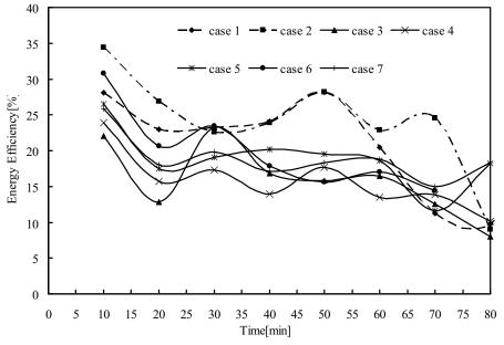
Figure 3.15 Energy efficiency profiles with respect to elapsed time in different case (F-bed)
