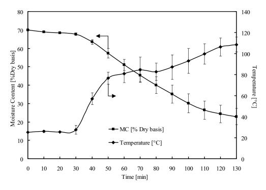
Figure 4.9 Temperature and moisture variations versus elapsed times in case drying using CMCB ( $T_1$ = hot air 70 °C)( case 6:Top feed)
