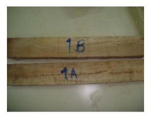
Sample after dried with Combined Multi-Feed Microwave -Convective Air and Continuous Belt System (CMCB)
