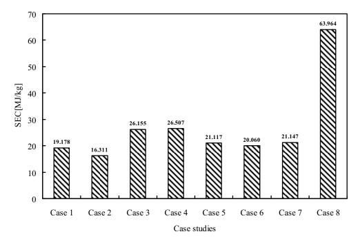
Figure 3.13 Variations in specific energy consumption in different case (F-bed)
