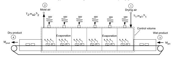
Figure 4.3 Schematic of control volume representing drying process using Combined unsymmetrical multi-feed microwave and hot air-continuous belt system (CMCB)
