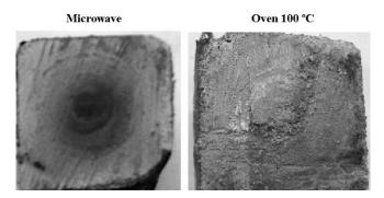
Fig. 7. Comparison of heat pattern in the specimens dried by microwave and oven at  $100\,^{\circ}\text{C}$
