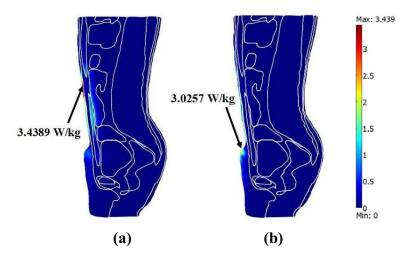
Fig. 5.9 SAR distribution in the human body (W/kg) exposed to the leakage power density of 5 mW/cm<sup>2</sup> at the frequencies of (a) 915 MHz (b) 2,450 MHz
