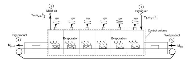
Figure 3.3 Schematic of control volume representing drying process using a combined multi-feed microwave-convective air and continuous belt system (CMCB)
