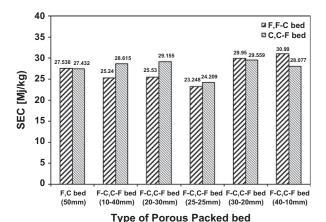
Fig. 17. Variation in specific energy consumption under microwave and convective drying at drying time 360 min.
