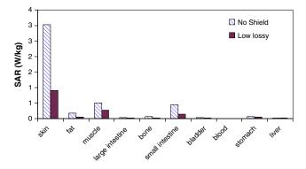
Fig. 12. Comparison of the maximum SAR in human organs of the unshielded and shielded human model at the frequency of 2450 MHz.
