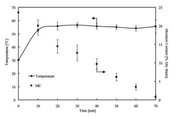
FIG. 6. Temperature and moisture variations versus elapsed times in case drying using CMCB ( $T_1 = 70^{\circ}$ C) (case 4, C-bed).
