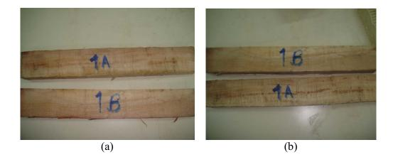
Figure 4.18 (a) Parawood pake before drying (b) Parawood pake after drying (CMCB)
