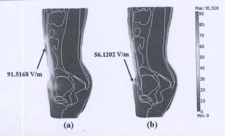
Fig. 8 Electric field distribution in human body (V/m) exposed to the leakage power density of 5  $\,$  mW/cm² at the frequencies of (a) 915 MHz and (b) 2450 MHz
