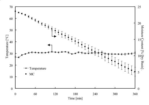
Figure 3.8 Temperature and moisture variations versus elapsed times in case using a convective drying ( $T_1$ = 70 °C)( case 8,C-bed)
