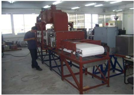
Hand on for a Combined Multi-Feed Microwave - Convective Air and Continuous Belt System (CMCB)
