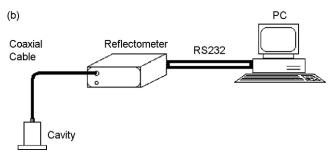
Fig. 2. Portable dielectric measurement (network analyzer).
