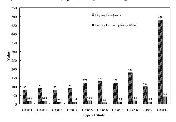
Figure 4.14 Variations in drying time and electrical energy consumption in different case
