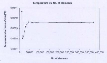
Fig. 5 Grid convergence curve of the 2D model
