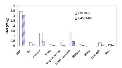
Fig. 5.16 Comparison of the maximum SAR in human tissues at the frequencies of 915 MHz and 2,450 MHz
