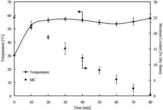
FIG. 7. Temperature and moisture variations versus elapsed times in case drying using CMCB ( $T_1 = 70^{\circ}$ C) (case 4, F-bed).
