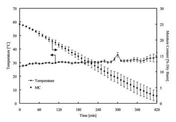
FIG. 9. Temperature and moisture variations versus elapsed times in case using convective drying ( $T_1 = 70^{\circ}$ C) (case 8, F-bed).
