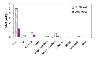
Fig. 6.12 Comparison of the maximum SAR in human organs of the unshielded and shielded human model at the frequency of 2,450 MHz
