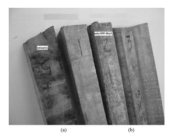
**Fig. 8.** Comparison of the quality of specimens dried by microwave (a) and oven at  $100\,^{\circ}\text{C}$  (b).
