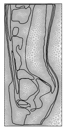
Fig. 4. A two-dimensional finite element mesh of human cross section model.
