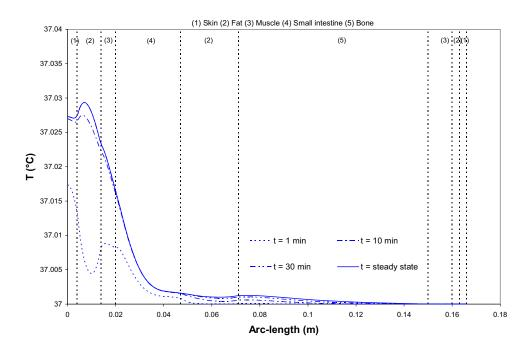
Fig. 5.11 Temperature distribution versus arc-length of the human body at various times exposed to the electromagnetic frequency of 915 MHz at the leakage power density of 5  $\,\mathrm{mW/cm^2}$
