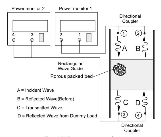
Figure 1.5 Microwave power measuring
