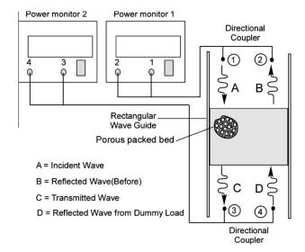
Fig. 4. Microwave power measuring.
