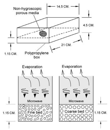
Figure 3.2 Schematic of drying sample (Porous packed bed)
