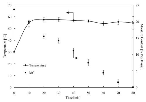
Figure 3.5 Temperature and moisture variations versus elapsed times in case drying using CMCB ( $T_1$ = 30 °C)( case 2,C-bed)
