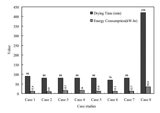
Figure 3.11 Variations in drying time and electrical energy consumption in different case (F-bed)
