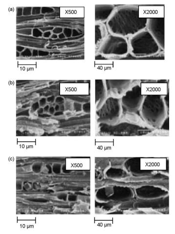
**Fig. 9.** Microstructure of specimen dried by different methods and conditions: (a) dried by microwave at 3200 W; (b) dried by microwave at 5600 W and (c) dried by oven at  $100\,^{\circ}$ C.
