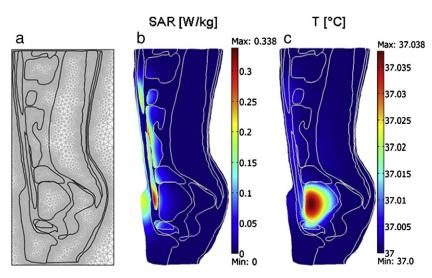
Fig. 8. Analysis of SAR and temperature distribution in the human model exposed to the microwave power density of 5 mW/cm² at the frequency of 300 MHz, (a) An initial finite element meshes of human cross section model (b) SAR distribution of the shieldless case (c) Temperature distribution of the unshield case.
