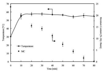
FIG. 5. Temperature and moisture variations versus elapsed times in case drying using CMCB ( $T_1 = 30^{\circ}$ C) (case 2, C-bed).
