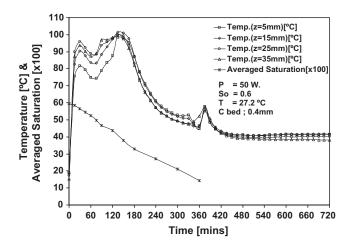
**Fig. 7.** Temperature and averaged saturation profiles with respect to elapsed time (C-bed, depth 50 mm).
