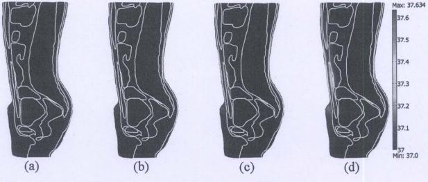
Fig. 19 Temperature distribution of human body exposed to the electromagnetic frequency of 915 MHz at t =1 min at various leakage power densities: (a) 5 mW/cm<sup>2</sup>, (b) 10 mW/cm<sup>2</sup>, (c) 50 mW/cm<sup>2</sup>, and (d) 100 mW/cm<sup>2</sup>
