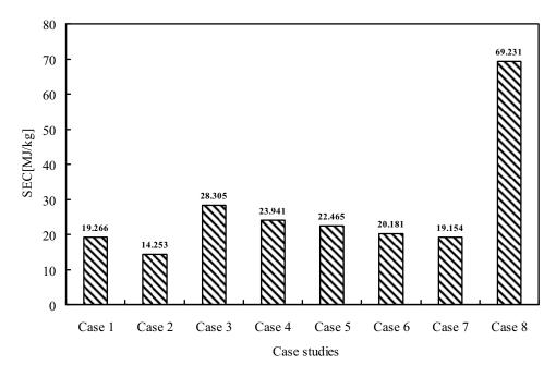
Figure 3.12 Variations in specific energy consumption in different case (C-bed)
