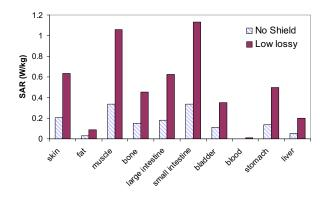
Fig. 6.11 Comparison of the maximum SAR in human organs of the unshielded and shielded human model at the frequency of 300 MHz
