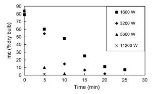
Fig. 3. Moisture profile versus elapsed times for different microwave power levels.
