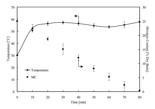
Figure 3.7 Temperature and moisture variations versus elapsed times in case drying using CMCB ( $T_1$ = 70 °C)( case 4,F-bed)
