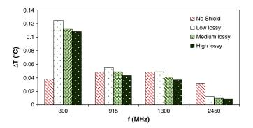
Fig. 10. Comparison of the maximum temperature increases in the human model at the frequencies of 300 MHz, 915 MHz, 1300 MHz and 2450 MHz.
