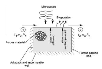
Fig. 5. Microwave and convective drying process.
