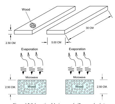
Figure 4.2 Schematic of drying sample (Parawood pake)
