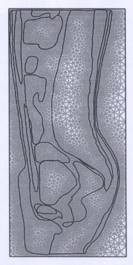
Fig. 4 An initial two-dimensional finite element mesh of human cross section model
