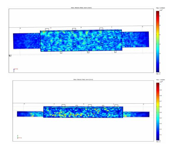
Figure 4.20 Computer simulation of electromagnetic field inside multi-mode cavity based on the concept of using the unsymmetrical multi-feed microwave
