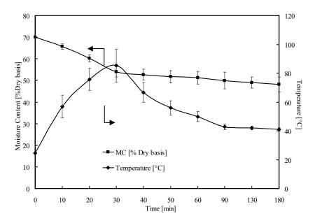
Figure 4.11 Temperature and moisture variations versus elapsed times in case drying using CMCB ( $T_1$ = hot air 70 °C)( case 8:Top feed)
