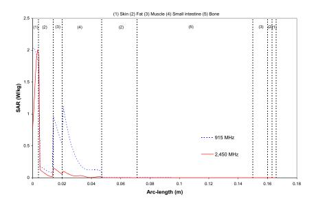
Fig. 5.14 SAR distribution versus arc-length of the human body exposed to the leakage power density of electromagnetic field at the 5 mW/cm<sup>2</sup>
