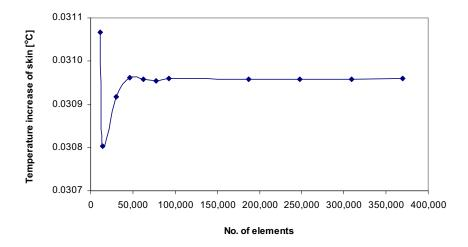
Fig. 6.5 Grid convergence curve of the 2D model
