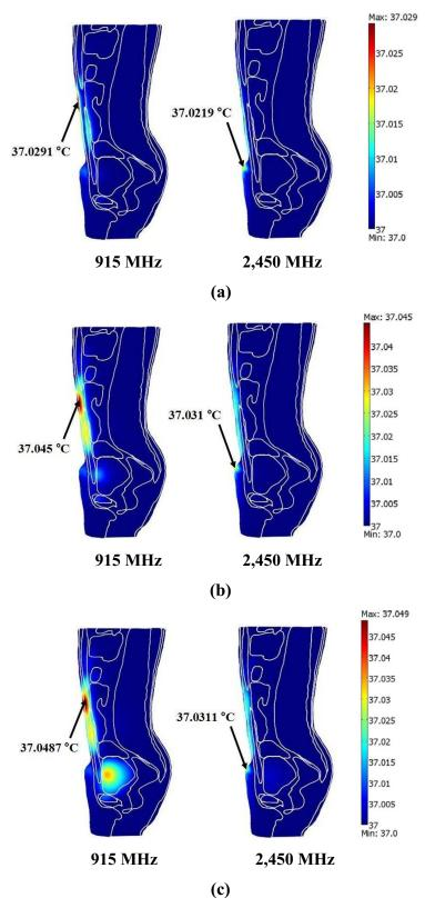
Fig. 5.10 The temperature distribution of the human body exposed to electromagnetic wave at the frequencies of 915 MHz and 2,450 MHz
