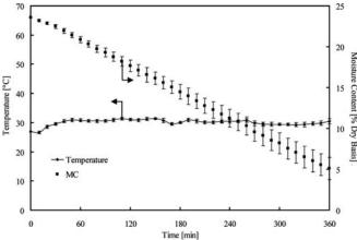
FIG. 8. Temperature and moisture variations versus elapsed times in case using convective drying ( $T_1 = 70^{\circ}$ C) (case 8, C-bed).
