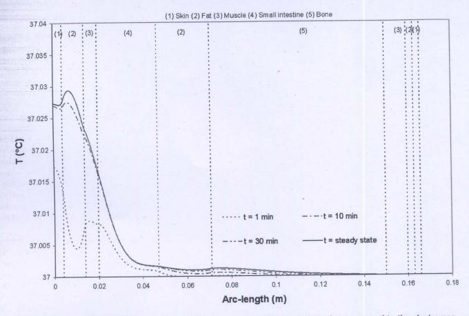
Fig. 11 Temperature distribution versus arc length of human body at various times exposed to the electromagnetic frequency of 915 MHz at the leakage power density of 5 mW/cm<sup>2</sup>
