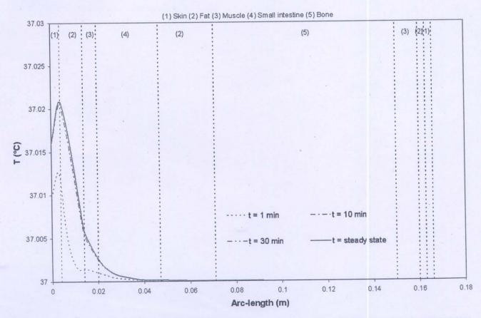
Fig. 12 Temperature distribution versus arc length of human body at various times exposed to the electromagnetic frequency of 2450 MHz at the leakage power density of 5 mW/cm²
