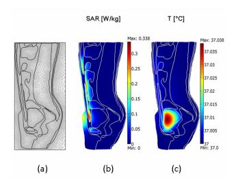
Fig. 6.8 Analysis of SAR and temperature distribution in the human model exposed to the microwave power density of 5mW/cm² at the frequency of 300MHz
