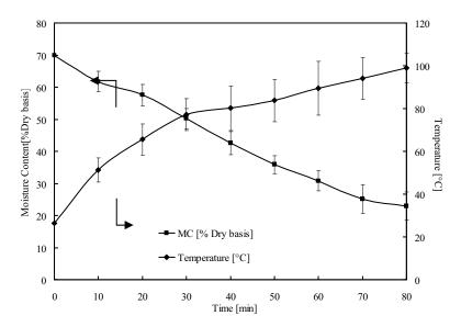
Figure 4.4 Temperature and moisture variations versus elapsed times in case drying using CMCB ( $T_1$ = 70 °C) (case 1:Top feed)
