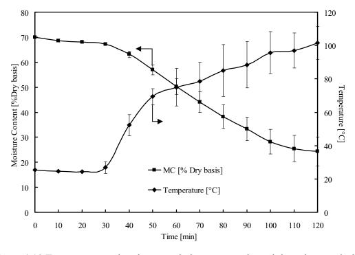
Figure 4.10 Temperature and moisture variations versus elapsed times in case drying using CMCB ( $T_1$ = hot air 70 °C)( case 7:Top feed)
