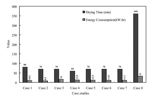
Figure 3.10 Variations in drying time and electrical energy consumption in different case (C-bed)
