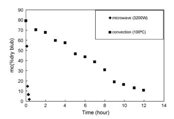
Fig. 4. Comparison of moisture profiles for different drying methods.
