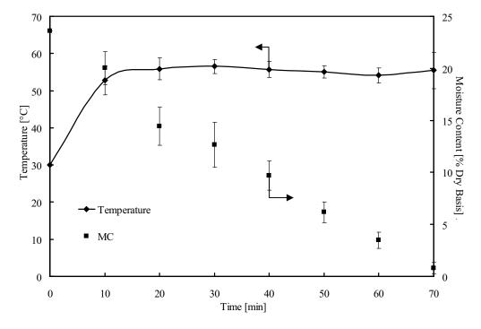
Figure 3.6 Temperature and moisture variations versus elapsed times in case drying using CMCB ( $T_1$ = 70 °C)( case 4,C-bed)
