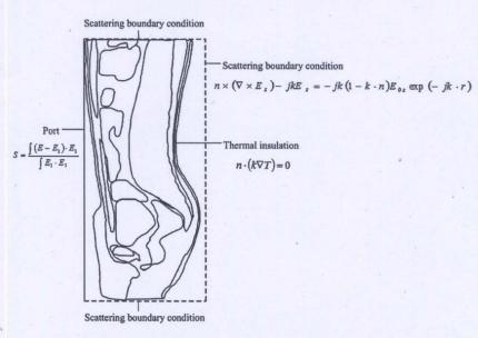
Fig. 3 Boundary condition for analysis
