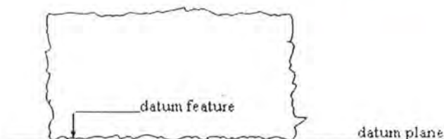
Figure 1. The mapping between a datum plane and a workpiece datum feature.
