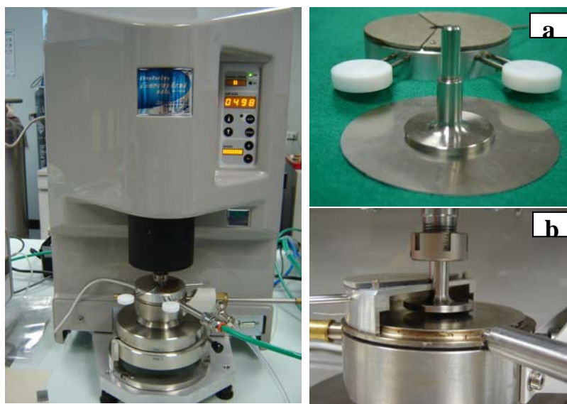
Figure 4.5 Bohlin Gemini HR nano Rotational Rheometer apparatus; (a) parallel plate geometry and (b) the gap between the plates.
