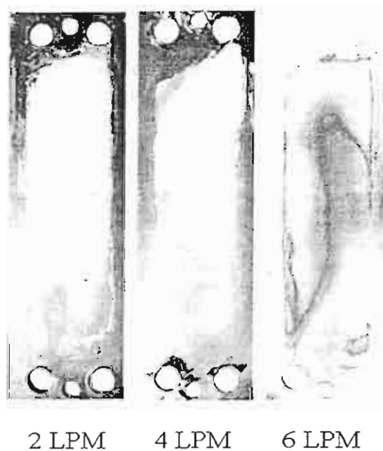
Figure 8 Photograph of the deposit on stainless steel plates at flowrate of 2, 4, and 6 LPM
