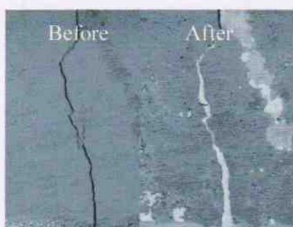
Fig. 3 Exposed surfaces of concrete specimens before and after charging ( \text{MgCl}_2 0.2 mol/L)
