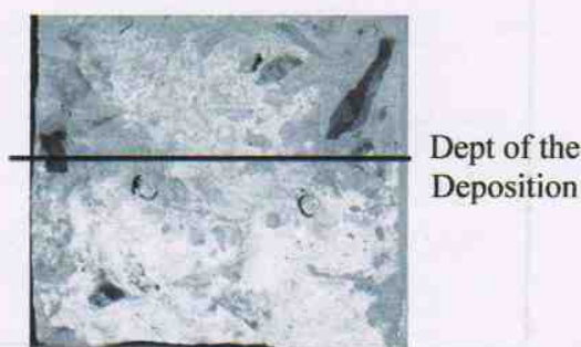
Fig. 4 Cross-section of electrodeposited concrete specimen ( \text{MgCl}_2 0.2 mol/L)
