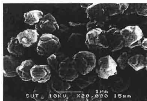
Figure 10 SEM image of zeolite Y synthesized from RHS with magnification of x20000
