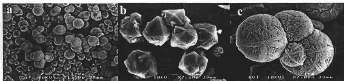
Fig.3. SEM image of NaY prepared from commercial silica source
