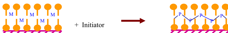
Figure 2. The admicellar polymerization process.
