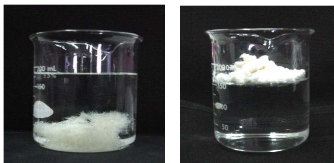
Figure 4. Flotation test of (a) untreated sisal fibers and (b) admicellar-treated sisal fibers.
