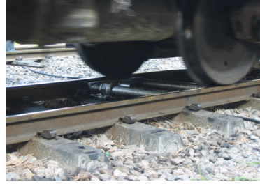
Figure 1. WEIGHWELL portable train weighing system
