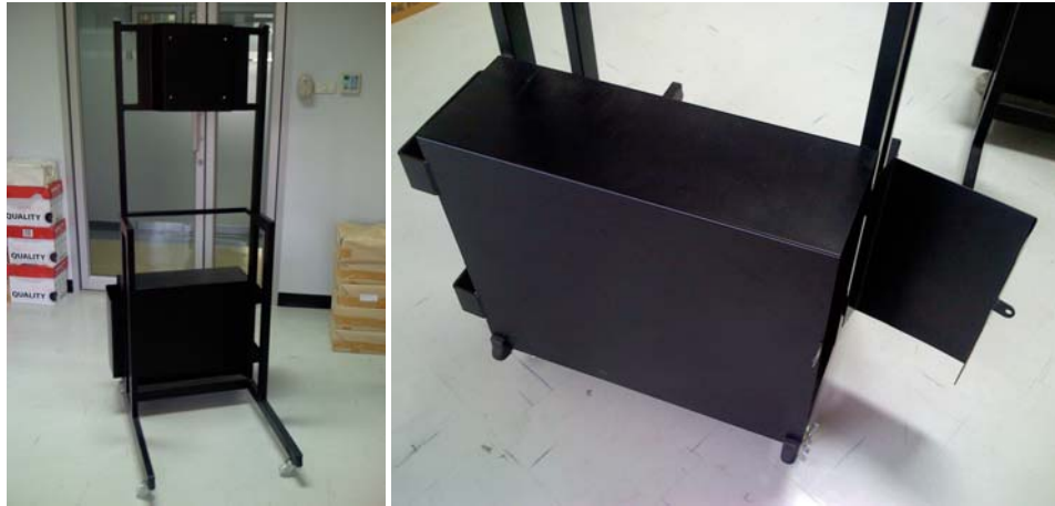
Figure 4.17 The first prototype stand with a locking compartment to enclose a PC. Unfortunately, the stand was not used for the user test of the system so no equipment were attached or installed on to the stand.
