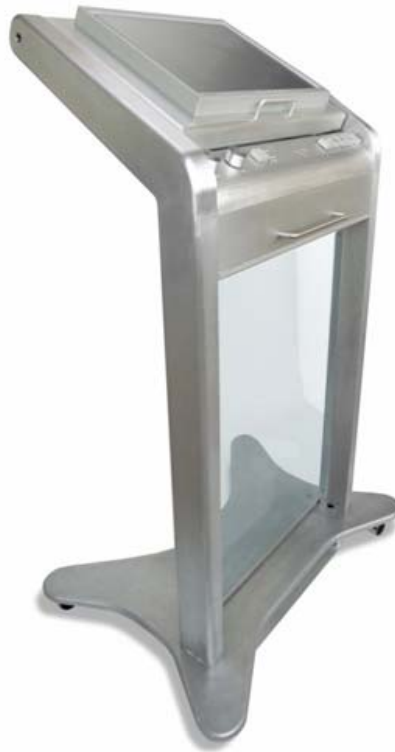
Fig. 4. The Convertible Podium's first operational prototype is CNC-machined from aluminum and acrylic panels and incorporates an onboard computer, WiFi, RFID, and custom sensing electronics.
