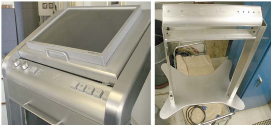
Fig. 12. The control strip and LCD screen installed, on the left; the control strip without buttons, the base and the side struts partially assembled, right.
