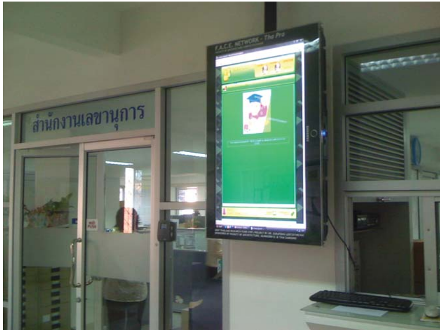
Figure 4.18 The redesigned FACE Network prototype. An integrated LCD display installed permanently to the ceiling in front of the administration office of the faculty of architecture in Tha Pra campus.
