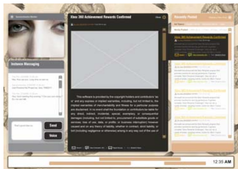
Figure 4.10 The first user interface designs balancing the screen percentage between content and features in a landscape orientation.
