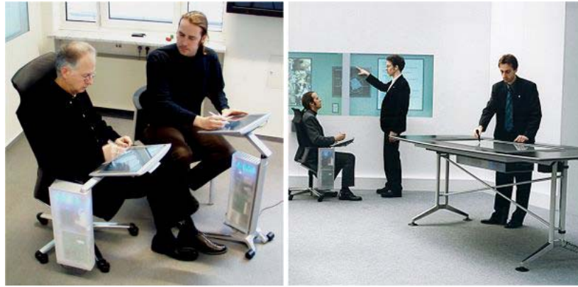
Figure 2.2 The CommChair (left), the DynaWall (middle), and Interactable (right) prototypes developed by Streitz et al. as a suite of roomware called “i-Land.”
