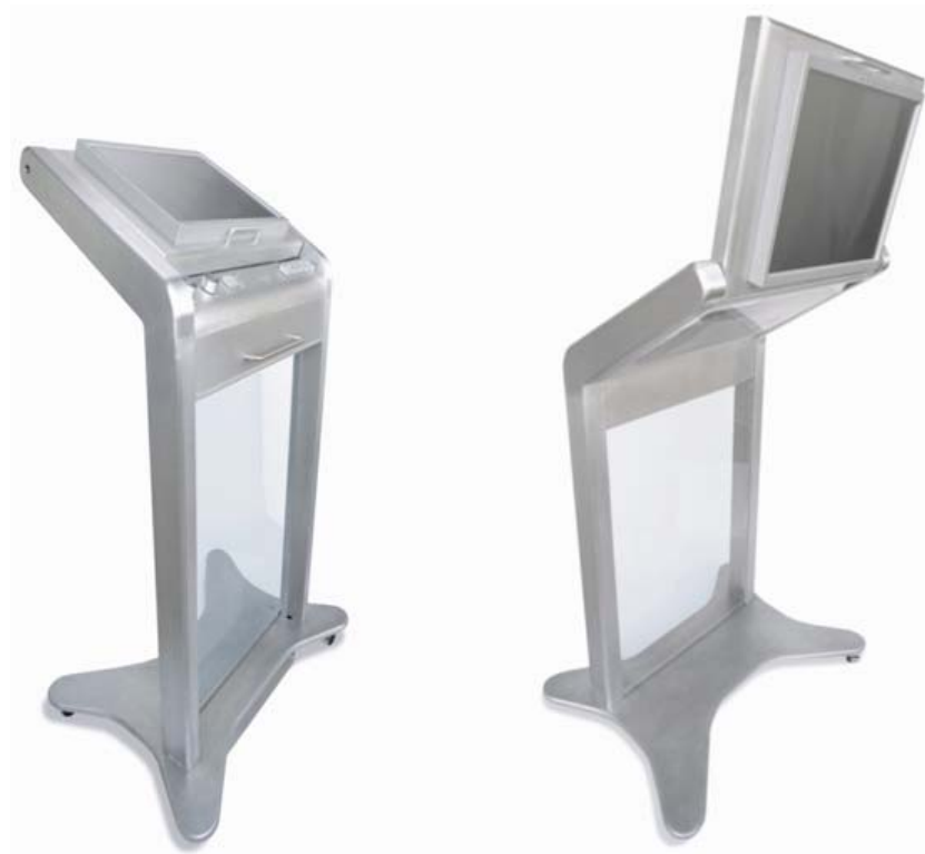
Fig. 5. The Convertible Podium's operational prototype upright in preparation for avatar mode. A motorized counterbalance system is installed within the aluminum strut along the left side of the Podium's faceplate, to handle the weight of the LCD monitor and its aluminum framing. In later designs, the monitor will be replaced with thinner lightweight displays such as e-paper or OLEDs
