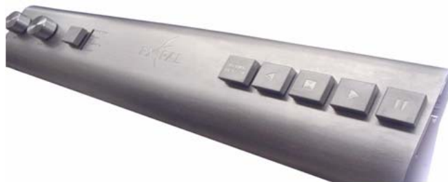
Fig. 9. The control strip features large, tangibly pleasing buttons and knobs that map clearly to software and environment controls. The control modules are modular and can be custom-designed for use with specific installations. In this case, software controls appear on the right; room controls are on the left
