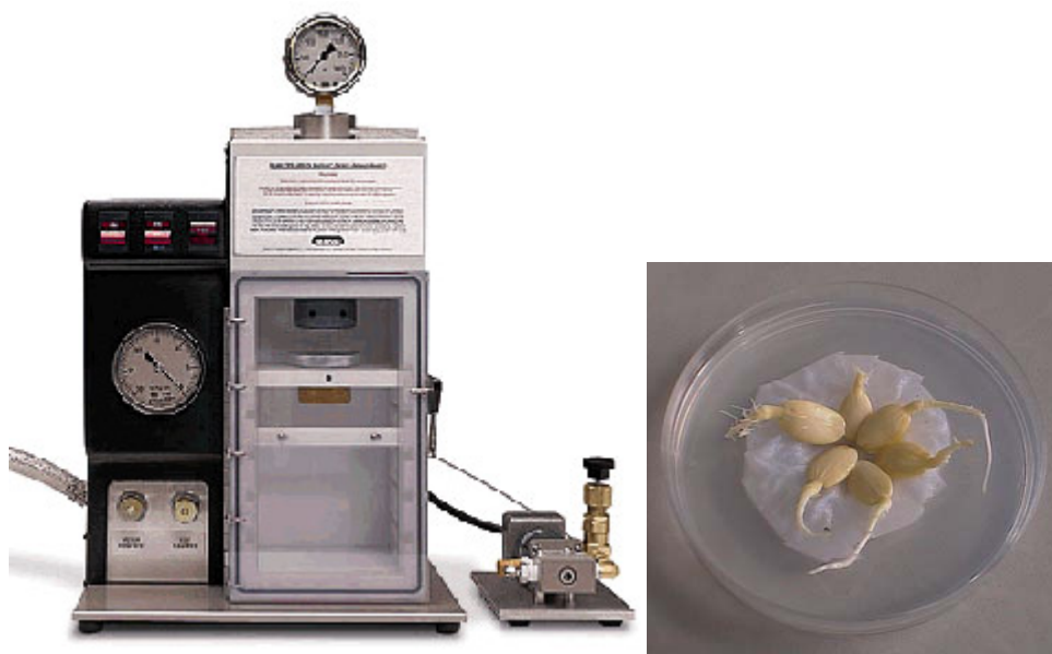
Figure 3 – Particle bombardment apparatus and zucchini seeds used for bombardment.
