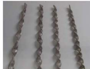
Fig. 2 Swirl generators with different twisted pitch number
