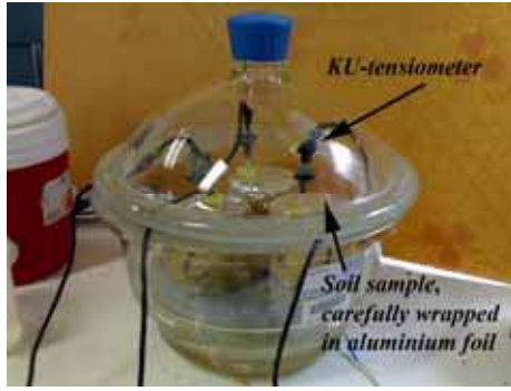
Figure 7. Experimental set-up for determining the soil-water retention curve using the tensiometer.
