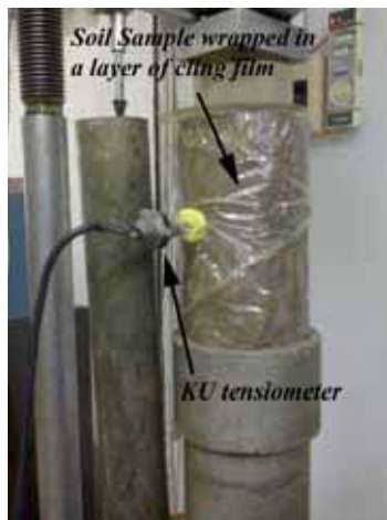
Figure 9. Experimental set up of the suction-monitored unconfined compression tests on soft Bangkok clay.
