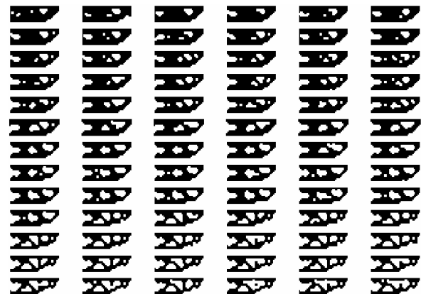
Figure 11. Topology results: 100 generations and 100 population size
