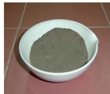
Fig. 1 Silt sample passing through No.200 sieve and retain on No.400 sieve
