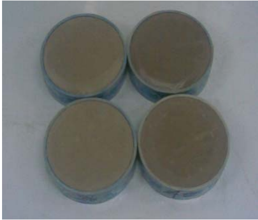
Fig. 3 The specimens with 63.3 mm in diameter and 20 mm height
