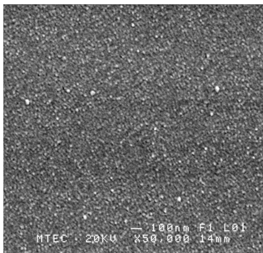
Fig.5 An SEM micrograph of the surface of 3-time dip coated TiO 2 film after calcination at 450 °C for 4 hrs.
