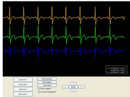
Fig. 3. The sample of simultaneously readings from one patient with our three-lead ECG device on a computer screen. From the top are the signals from Lead III, Lead II and Lead I.
