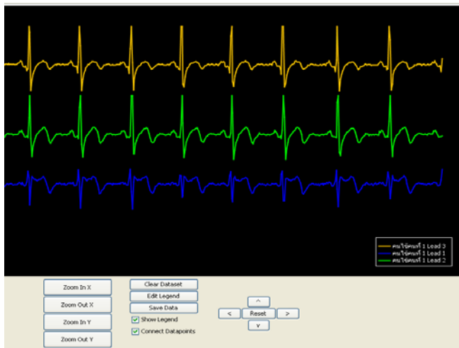
Fig. 6. The sample of simultaneously readings from one patient with our 3-lead ECG device on a computer screen. From the top are the signals from Lead III, Lead II and Lead I.
