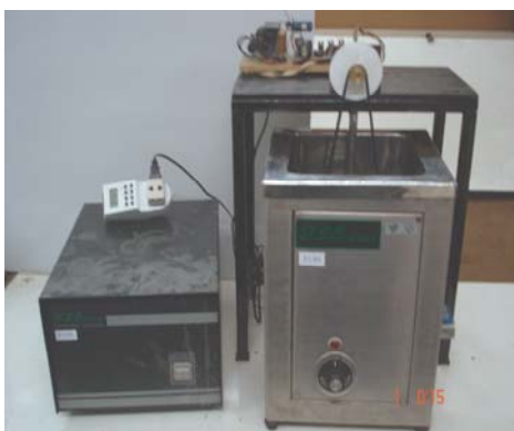
Figure 1. Fabrication of BZT powder using the ultrasonic ball-milling technique.
