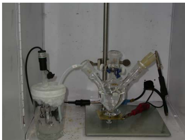
Figure 2.1 The electrochemical cell for cyclic voltammetric study.
