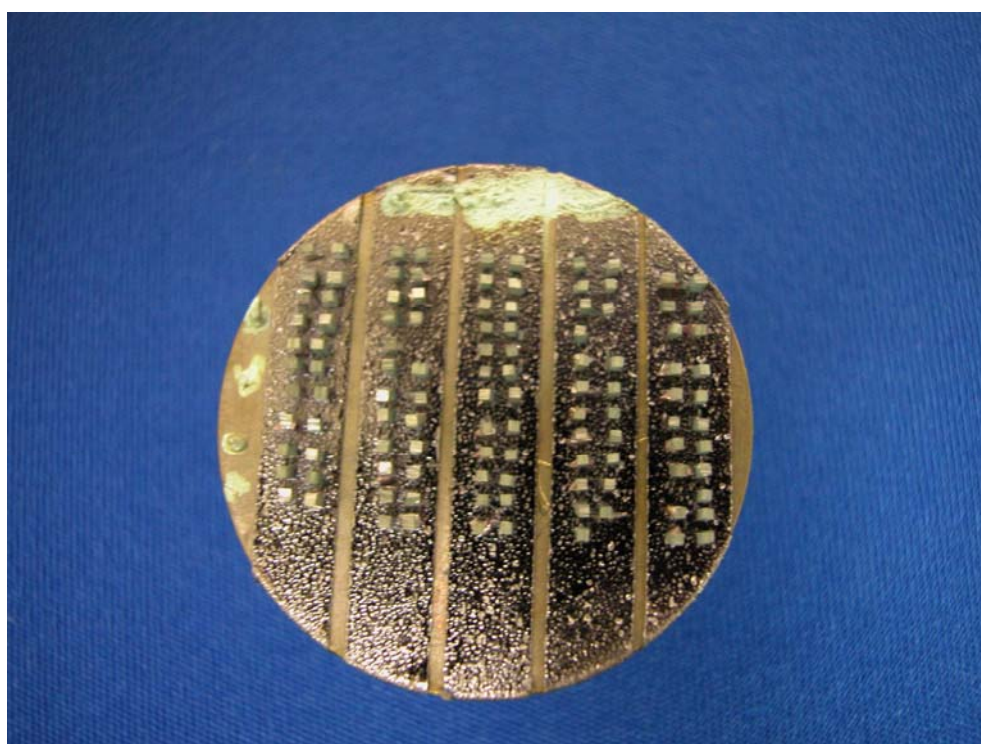
Figure 2.2 Fractured beams mounted on brass tablets and gold sputter-coated.
