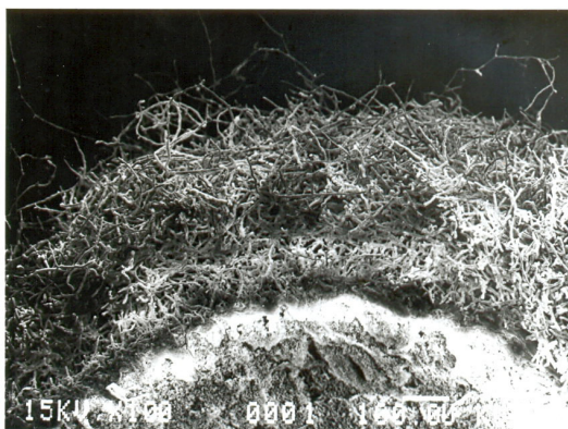
Fig. 2 SEM photograph of the cross section of chitosan immobilised bead.
