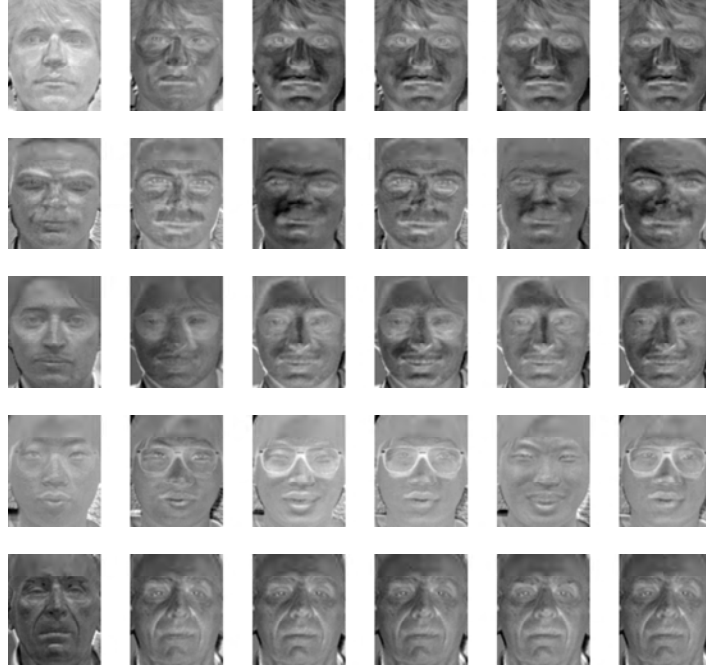
Figure 5. Samples of reconstruction images used for class-specific classification approach. The first images in the first column are the input testing images. Images of the second to the sixth columns are corresponding to the class-specific principal component analysis reconstruction. Note that all the images here are reconstructed using the eigen-domain based reconstruction approach.
