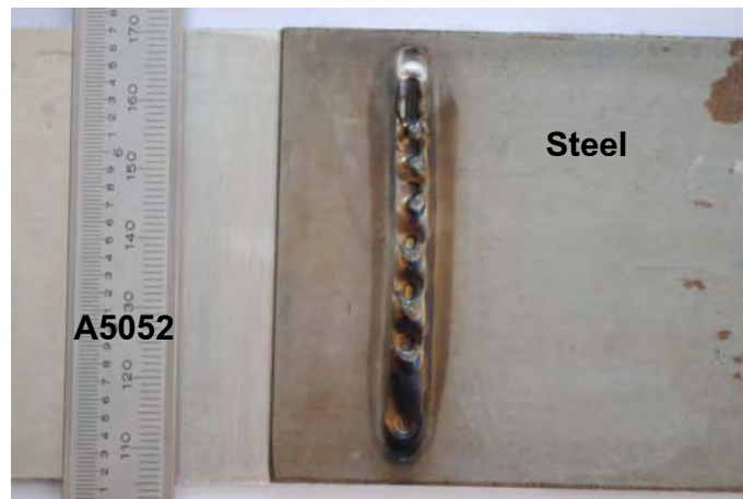
Fig. 3.25 Arc blow problems found in joint with 170 A of welding current, 0.6 m/min of welding speed and 3.2 mm of arc length.
