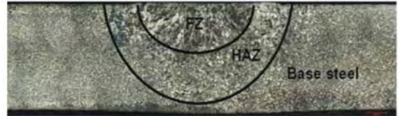
Fig. 2: The macrostructure of steel weld with electrical current of 45 ampere current and 0.65 m min -1 of welding speed
