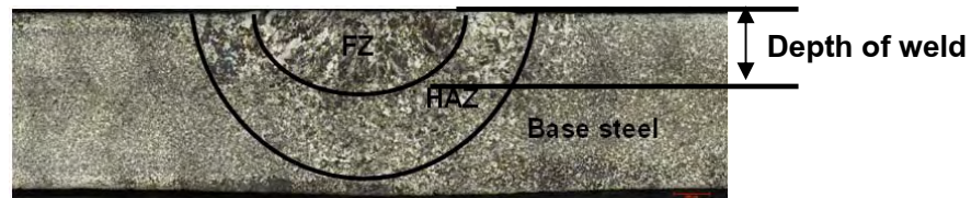
Fig. 3.2 Example of cross-sectional observation of steel after beading on the plate with 45 A of electrical current and 0.65 m/min of welding speed.
