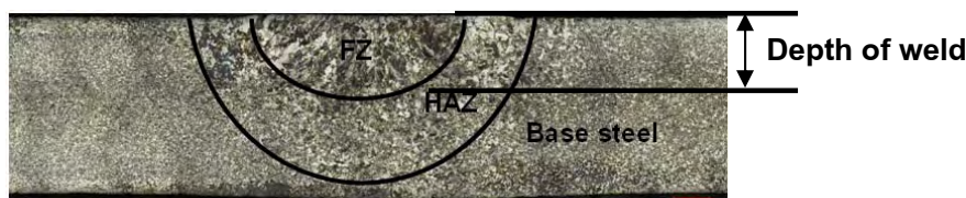
Fig. 2.14 Schematic of definition of depth of weld
