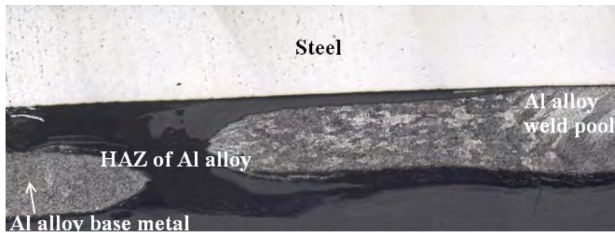
Figure 3.18 Fracture path of the joint between steel/A1100 obtained with 0.65 m/min of welding speed and 165 A of electrical current.
