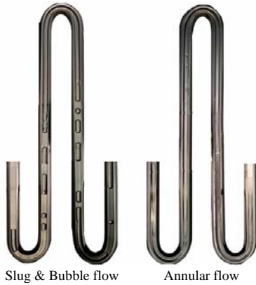
Figure 9: Internal flow patterns of HCLOHP with 50% filling ratio of water.
