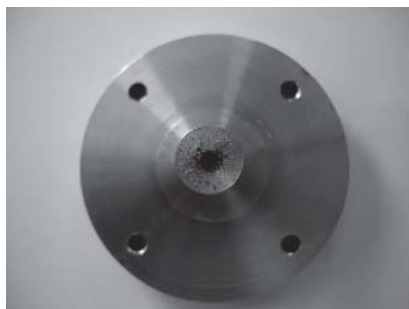
Figure 9. Photograph of typical particles collected on the impaction surface inside of the impactor.
