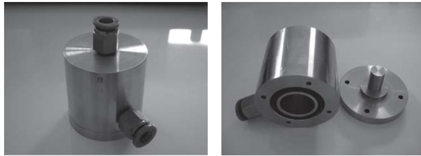
Figure 2. A picture of the submicron-sized particle inertial impactor.
