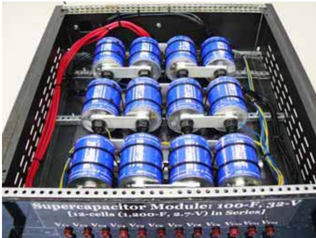
Fig. 9. Test bench of supercapacitor module of 100 F, 32 V.
