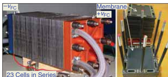
FIGURE 13 – PEMFC stack: 500 W, 40 A, and 13 V.
