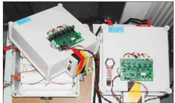
FIGURE 15 – Supercapacitor module: 292 F, 30 V, and 500 A.
