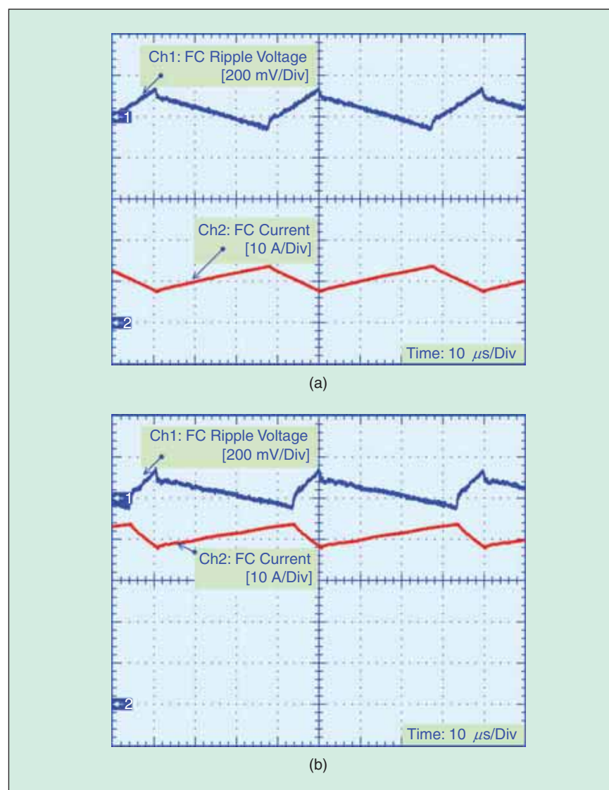
FIGURE 4– Switching characteristics of a 500 W PEMFC of 25 kHz at the FC current supply of (a) 10 A and (b) 40 A (rated current).
