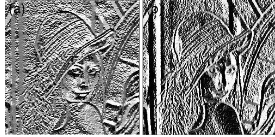
Fig. 3 Gradient orientation patterns of the Lena image: (a) n_x (b) n_y .
