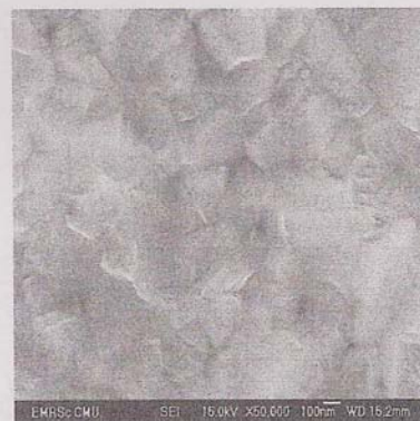
Fig. 2 Typical SEM micrograph of rutile \text{TiO}_2 thin films at temperature 700°C
